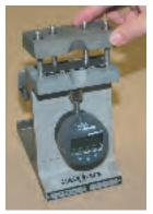
The Aero-Almen gage and aluminum strips provide a definitive measurement and quality control for the PMB process of the shuttles' solid rocket boosters. condition. The challenge now was how to quantify and control this degree of blast intensity.
