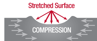
FIGURE 1-2 Compression Resists Fatigue Cracking
