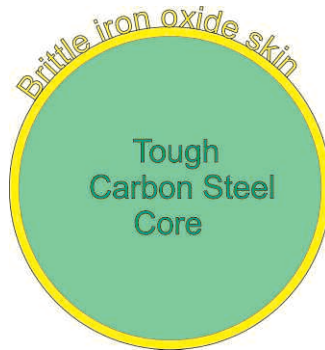
Fig.1 Section of spherical carbon steel shot particle.
