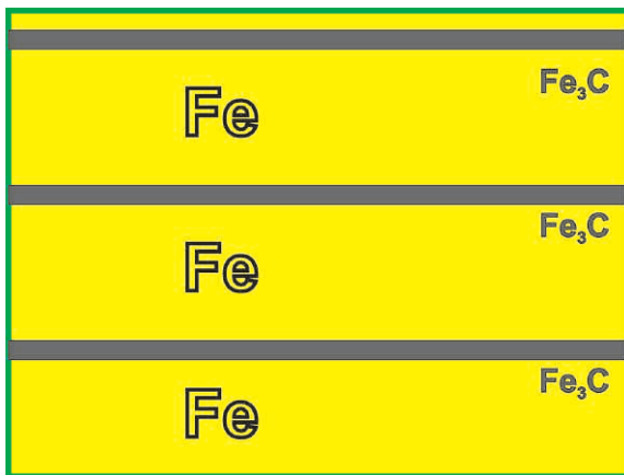
Fig.4 Schematic representation of "Pearlite" structure.
