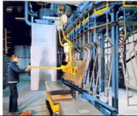
Blast cleaning system and handling equipment for blast cleaning sheet metal plates
