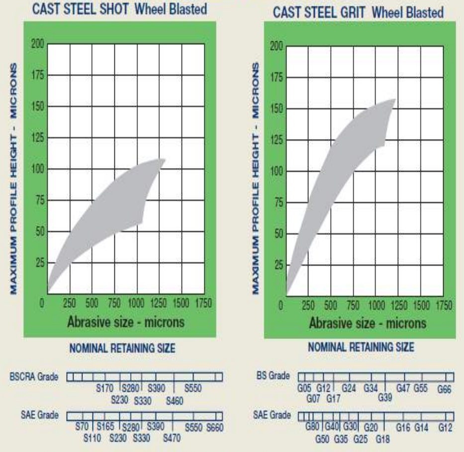
Plot of maximum profile height and nominal retaining size for airless wheel blasted abrasives Note: See previous page for other factors that affect surface profile.
