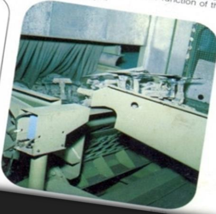
View from the loading end of the +GF+ Vibrating Conveyor Blast Cleaning Machine type VD-4. After the shake-out, the cooled castings are brought to the vibrating conveyor where a light beam barrier controls the function of the vibrating conveyor.
