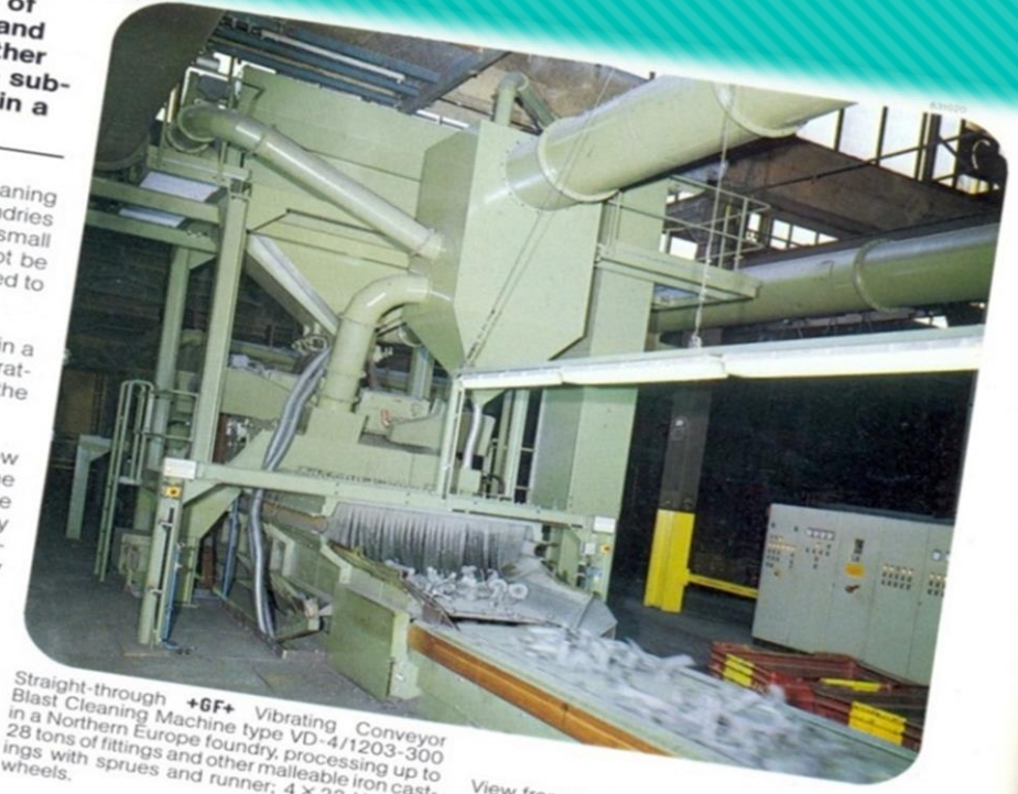
View from the loading end of the +GF+ Vibrating Conveyor Blast Cleaning Machine type VD-4. After the shake-out, the cooled castings are brought to the vibrating conveyor where a light beam barrier controls the function of the vibrating conveyor.
