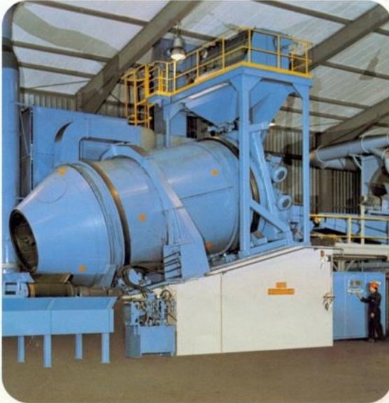
DT-2 Shot blast machine receiving the castings from 2 moulding lines and cooling drums.
