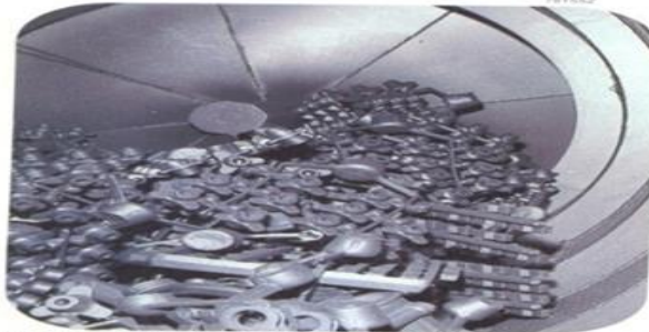
Blast area in the +GF+ Straight-through Barrel blast machine type DT with clusters of nodular iron castings.
