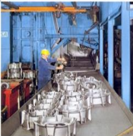
Even large parts can be perfectly shotblasted
